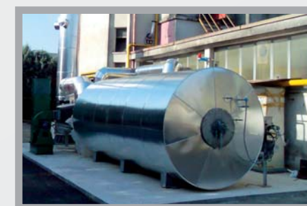
Recuperative Thermal Oxidizer with integrated heat exchanger
