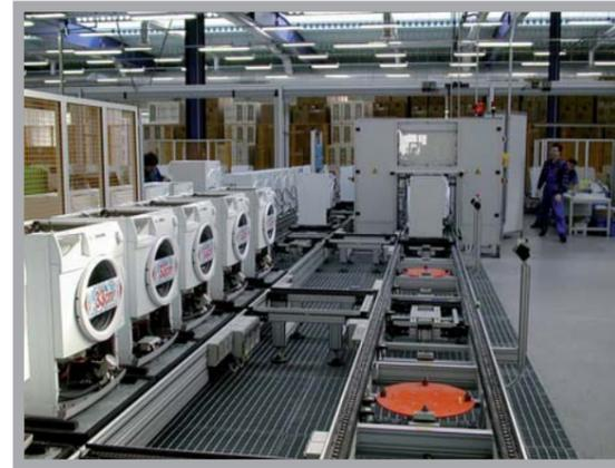
On floor conveyors with flying roller chains or flat chains allow us to develop flexible systems. They are used every time it is necessary to handle and work with products transported on pallets in a fast, precise, reliable, silent way achieving series or parallel working areas.
