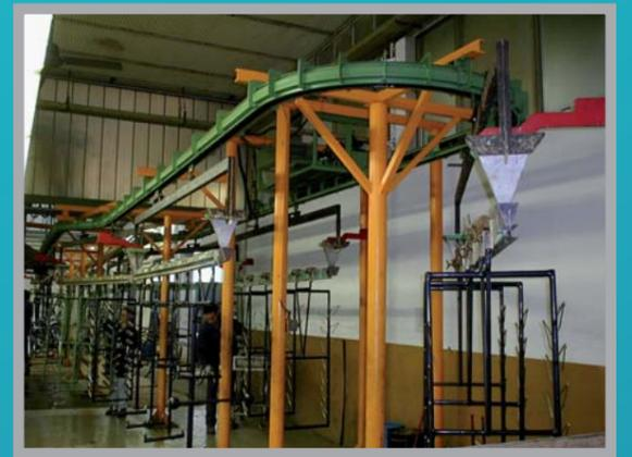
Overhead and up-turned monorail conveyors can solve the simplest conveyance and storage problems by connecting two or more similar-paced workstations.
