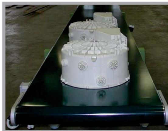
Belt conveyors make it possible to create light transport systems, having the flexibility and modularity characterising Movin products. They are used every time it is necessary to handle products without pallets, in a precise, reliable, fast and noiseless way.
