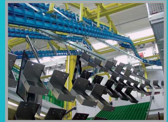
Power & Free Conveyors are systems able to solve very complex problems of mechanical handling, such as interconnection between two or more working areas which are operating according to different timing.
