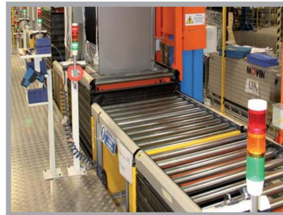
Rollers conveyors are mainly used when it is necessary to handle and work products without supporting pallets or polystyrene and/or paperboard bases or products gathered on wood pallets.
